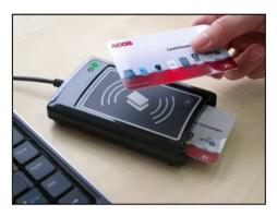
ACR1281U-C1 DualBoost II is the second generation of ACS's ACR128 DualBoost Reader. It is a dual interface reader that can access any contact and contactless smart cards following the ISO 7816 and ISO 14443 standards. ACR1281U-C1 enables one to conventionally integrate separate and independent applications for contact and contactless technologies into one device and one card.
